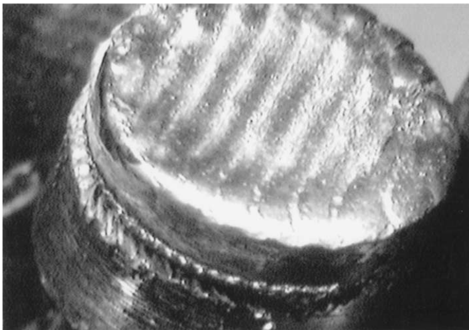
Figure 7 A view of a contact tip with an Mo-Ni surface layer; visible paths after the alloying process using an Nd: YAG laser (A type lasers).
